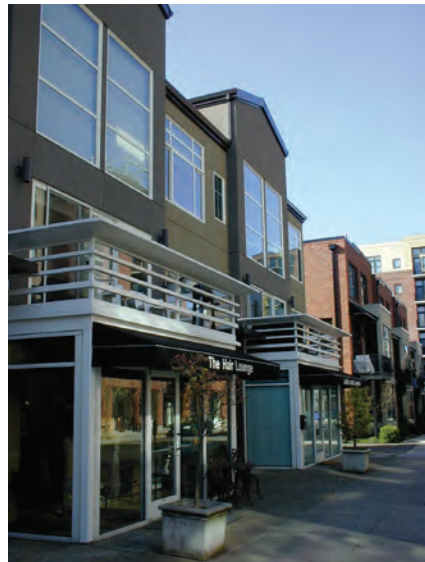
Use of horizontal modulation to emphasize size of units in residential buildings
